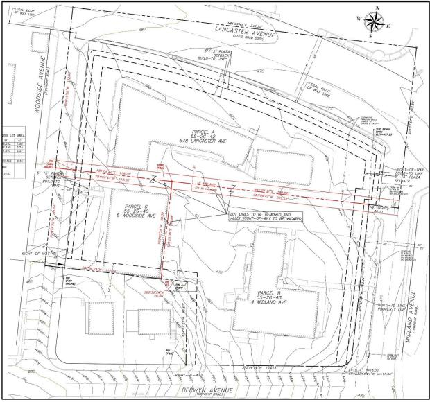
Site Plan Detail, Sheet 3 – Lot Consolidation Plan
